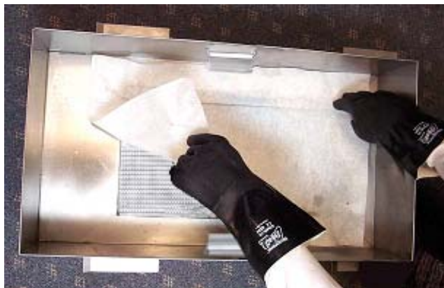
Remove and discard old filter paper.
