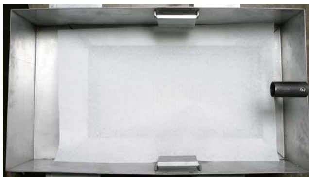
Proper filter paper placement.
